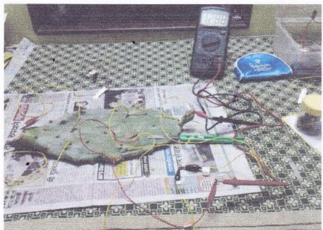
6) Prickly Pear plant with Zn-Al electrodes indicating 1.288V output on DMM
